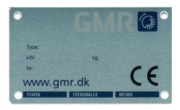
The machine is equipped with a riveted information plate/number plate. The engraved number in this plate is unique for the actual machine, and the factory will always be able to trace the machine if this number is given.
