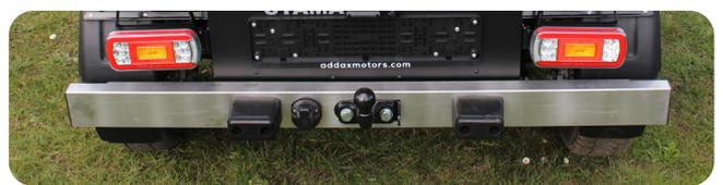
Trailer hitch (only with 12.5:1 transmission / 55 km/h)
