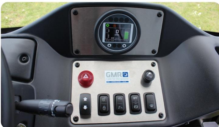
Dashboard with control panels: forward/reverse switch, switch for warning light, for locking/unlocking the doors, 2-stage drive switch fast/slow, up-hill start assist, windshield wiper on / off, washer fluid and cigarette lighter
