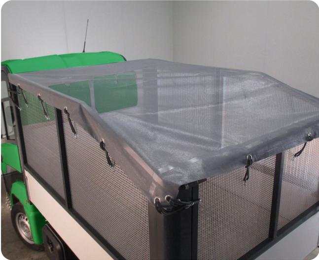
Water and air permeable tarp cover on high drop-sides with net
