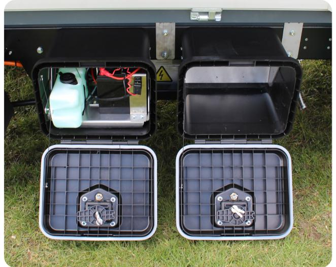
Left box: water tank for front window wiping / washing system and 12V battery for the use of light, heated front window etc.
