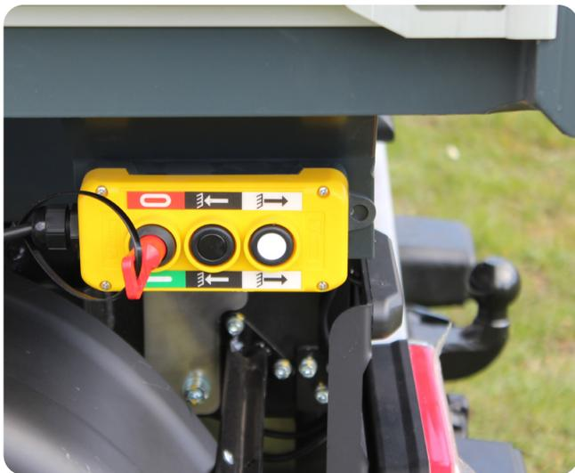
Control box for hydraulic tipper, with key
