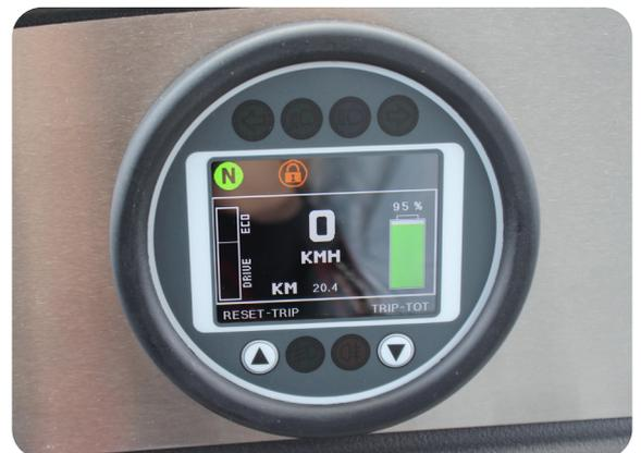
Control display with mileage display, operating hours counter, battery charge display and error codes
