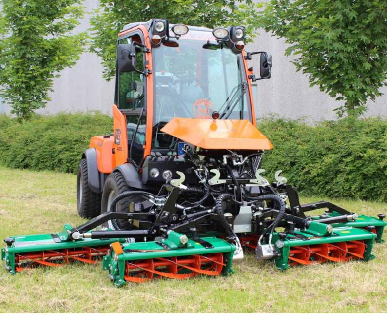
The rotary mowers are offered with either rear or side discharge (for collection). The side dischage mowers are available from 1,2 to 4,0 meters and offer perfect distribution of grass.
