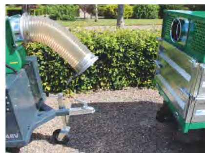
Simple mounting of towed unit and discharge hose
