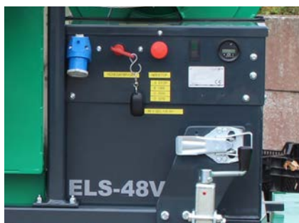
Manageable and easily accessible control panel with i.a. 220V charging socket
