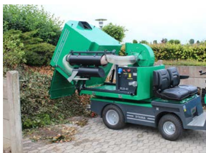
Easy emptying, as both tip and door are hydraulic on the collection box
