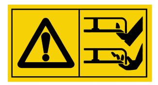
Warning of crushing hazard:
